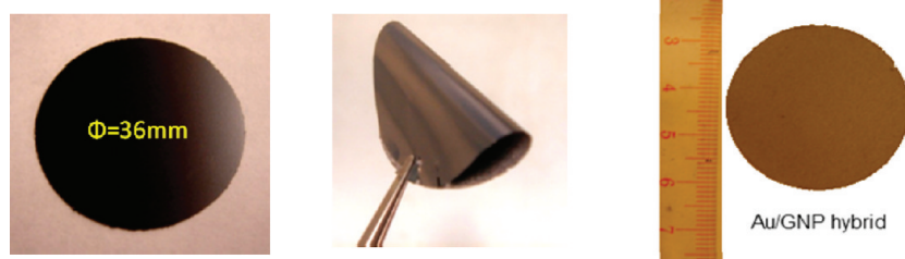
Figure 3. Photos of the as-made GNP paper showing flexibility and mechanical robustness under bending and the Au/GNP hybrid sample used for thermal diffusivity measurement (1 in. diameter).
